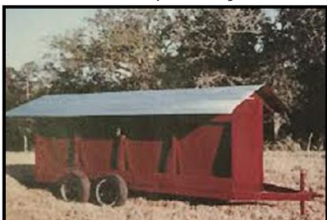
Model 16W: 9000 lb / 224 cu ft capacity 16' L x 4' W x 7' H
